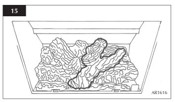
5.6 Carefully insert the front coal retainer into the front panel of the firebox. Take care not the scrape/damage the logs. This coal retainer sits in two brackets. Ensure it is fully inserted, leaving approximately a 4 mm gap between the firebox ledge and the bottom of the coal retainer.
